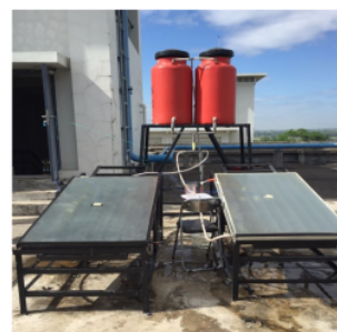
Fig. 2. SWH system using V-shaped absorber plate: on the left, with PCM storage and on the right, without PCM storage
